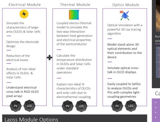
We offer three modules with Laoss: Optical, Electrical and Thermal. The optical and electrical modules can be purchased separately. The thermal module requires a license of the electrical module and considers electro-thermal coupling.
