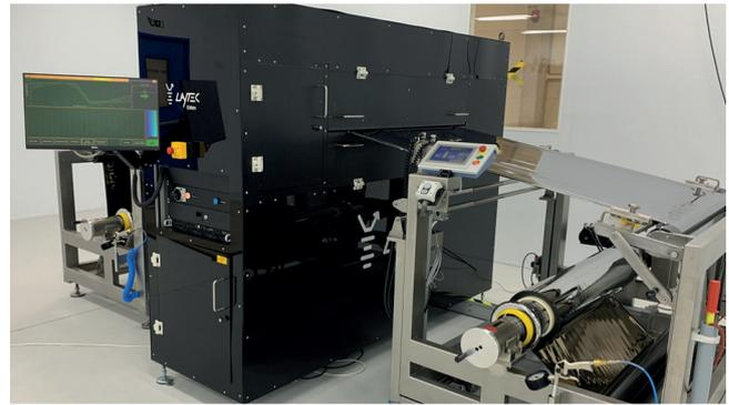
Fig. 4 Photograph of an ILMetro R2R metrology setup for the fully automated quality control of entire roll pairs by means of reflectance and transmittance spectroscopy as well as eddy current measurements for determining the sheet resistance of metallic and TCO layers.
