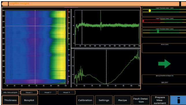
Fig. 3 Typical view of the graphical user interface of LayTec's metrology software displaying the spectrogram of the current deposition campaign (left), the thickness evolution (upper right) as well as the selected spectrum (lower right). Additionally, fields for statistical process control are displayed.
