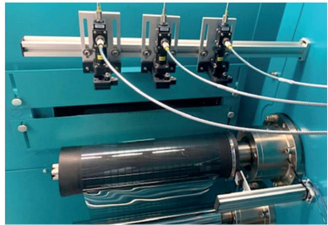
Fig. 1 Photograph of a 3-head Flames setup in the R2R-deposition line of OET for in-line monitoring of the film thickness of organic layer stacks on flexible substrates.
