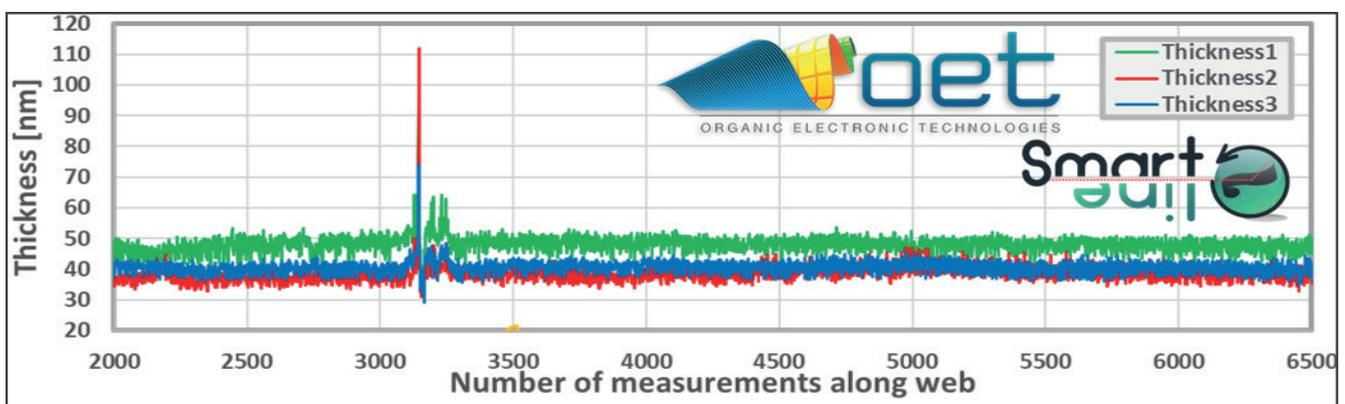
Fig. 2 In-line thickness monitoring data as obtained with a 3-head Flames system on R2R-deposited electron transfer layers (ETL) in a PET / ITO-metal-ITO (IMI) stack configuration.
