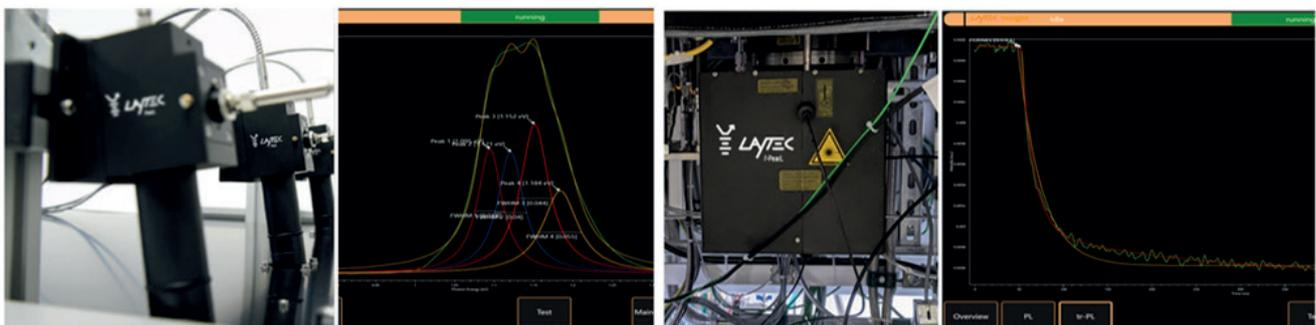
Fig. 5 Left: Production-integrated in-line Pearl metrology system for spectral photoluminescence measurements and exemplary data. Right: Vacuum-integrated combined Pearl/t-Pearl setup for in-vacuo and exemplary transients for time-resolved photoluminescence measurements are shown.
