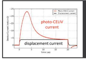
RC-effects are superimposed on the device current and can significantly disturb transient experiments.
