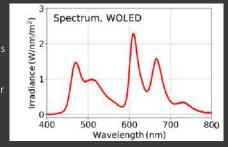
The use of a calibrated spectrometer allows to quantify the absolute spectral and integrated irradiance, luminance and current efficacy as well as CIE and color temperature.
