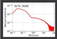
Deep-level transient spectroscopy (DLTS) is a measurement to characterize traps inside a diode.
