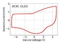
Displacement current measurement (DCM) with cycles of up and down voltage ramps
