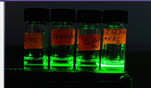
Tyndall effect studies carried on the as labelled perovskite precursor solutions after filtration with a 0.45μm nylon filter, prepared from different MAI powders (as labelled from left to right): 'old MAI 1x RC', 'old MAI 3 x RC', 'New MAI no additive(0wt% additive) and 'comm.MAI'
